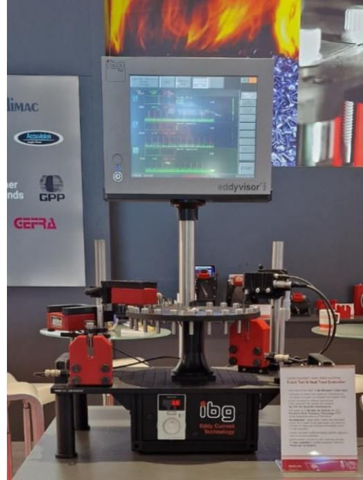
Dynamic structure test & crack detection
